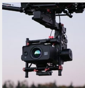
Gas leaks visualization
