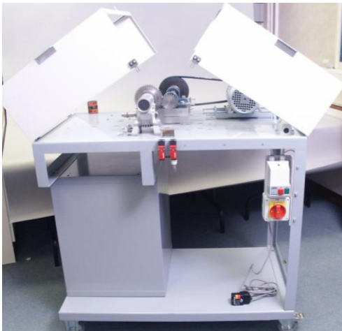
Removable guards for ease of practical exercise construction with safety interlock
