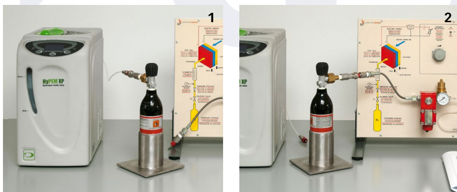
Feeding the fuel cell with hydrogen from the storage tank H2-300 (image 2), previously fed by the PEM Electrolyzer HG-300 (image 1)
