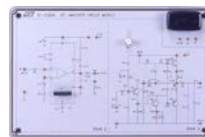
KL-23006 OTL Amplifier Circuit
